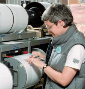
When an earthquake occurs, the vibrations are detected by seismographs at different locations. These multiple measurements confirm the detection of an earthquake.
