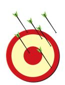
Low accuracy: The cluster of arrows is on one side of the target.
