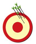
Low accuracy: The cluster of arrows is on one side of the target.
