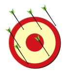
High accuracy: The center of the cluster is close to the center of the target.
