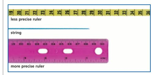
The instruments you used had different precisions. A ruler that is marked in tenths of a centimeter lets you make more precise measurements than one marked only every centimeter. The more finely marked ruler is considered more precise.
