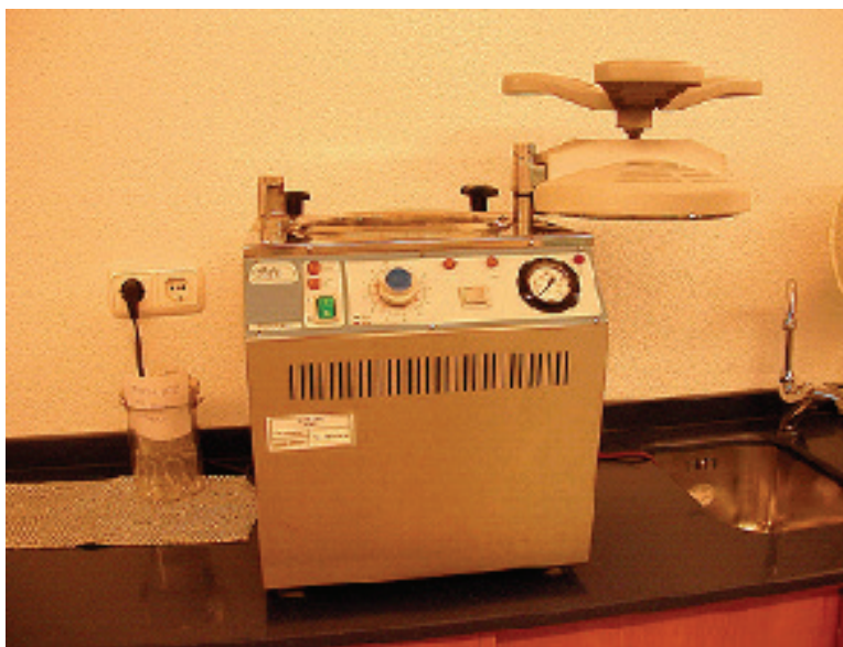
Figure 1.35: A worktop autoclave. Autoclaves commonly use steam heated to 121^{\circ}\text{C} ( 250^{\circ}\text{F} ), at 103 kPa (15 psi) above atmospheric pressure. Solid surfaces are effectively sterilized when heated to this temperature. Liquids can also be sterilized by this process, though additional time is required to reach sterilizing temperature. (24)
