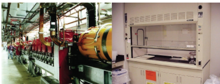
Figure 1.28: Different fields of science need different types of equipment, such as the particle accelerator at left, found in a physics lab, and the fume hood, at right, found in chemistry labs, but also sometimes in biology labs. (10)
