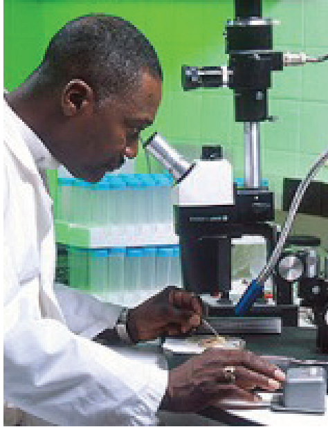
Figure 1.31: This scientist is using a stereo microscope, which is a light microscope with two ocular lenses (the microscope lens that is closest to the eye). The microscope is fitted with a digital imaging device that can take digital photos of what the researcher sees. (37)
