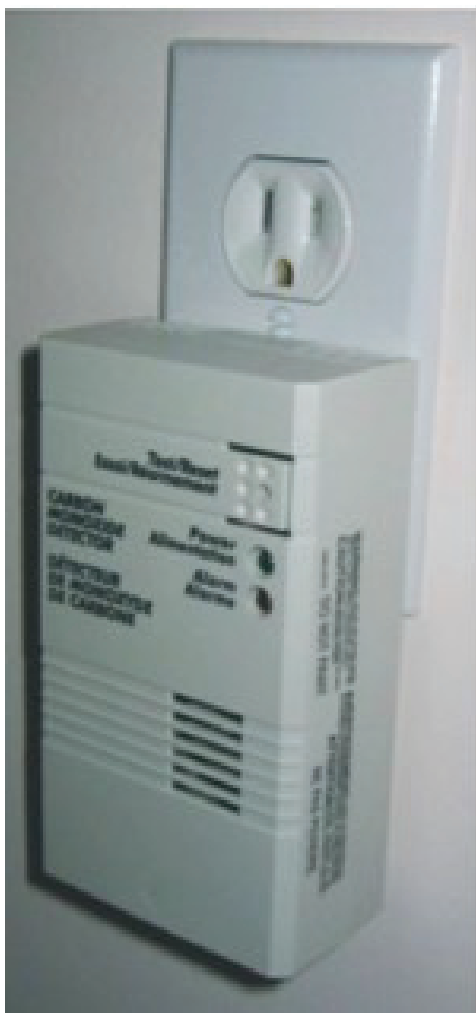
Figure 24.15: Home carbon monoxide detector (13)
