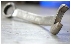
This wrench, found in a car shop in Malaysia, has been subjected to much abuse and is clearly showing signs of age. In its current condition, signs of rust shows that, at a molecular level, its metallic bonding is not perfect and the bending indicates that the original <a href="mailto:crystalline structure">crystalline structure</a> is altered.
